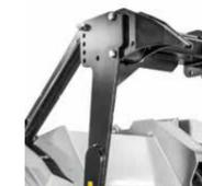
**2** **Mechanical/hydraulic push frame** guides and pushes material away from carrier
