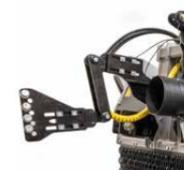
**1** **W style self aligning device between PTO drive shaft/gearbox** allows the mulcher to work at several angles without damaging the PTO
