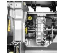
**4** **Standard hydraulic clutch transmission (UMH/S)** protects the transmission at PTO engagement for smooth starting and improves machine performance
